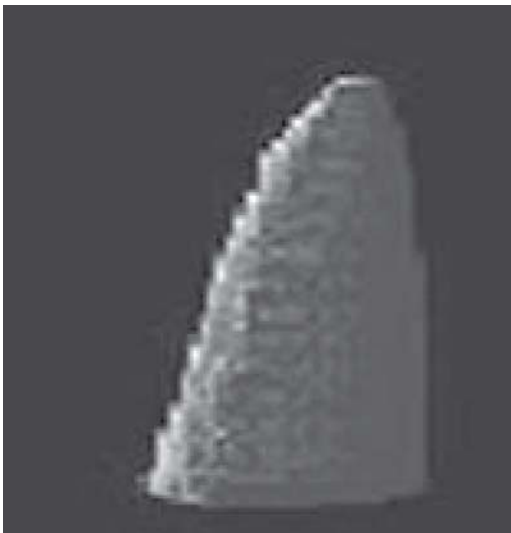
Fig. 7 Tomographic image showing asymmetric morphology. Experiments performed at 750 °C during 6 h.
