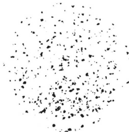
Fig. 5 Horizontal slice binary image. Dark regions correspond to the \text{Ni}_3\text{Si}_2 phase.
